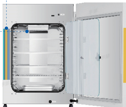
The three-layer thermal stability design of the water jacketed interlayer
