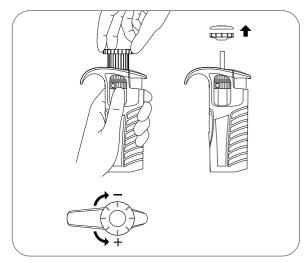
**NOTE:** Before calibration, in the Discovery Comfort and Discovery Pro lines, always remember to lock the volume using the lock function and for the Labmate Pro and Optipette hold the calibration knob.
